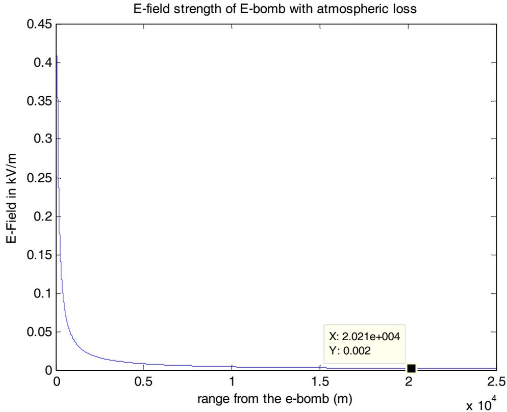
Figure 36. Low-tech E-bomb lethality range for KIM-1 microprocessor
