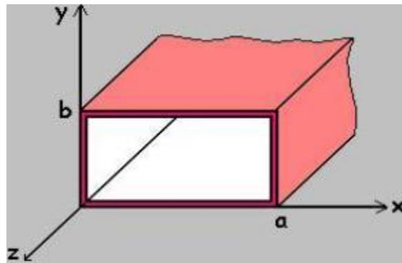
Figure 17. Waveguide dimensions
