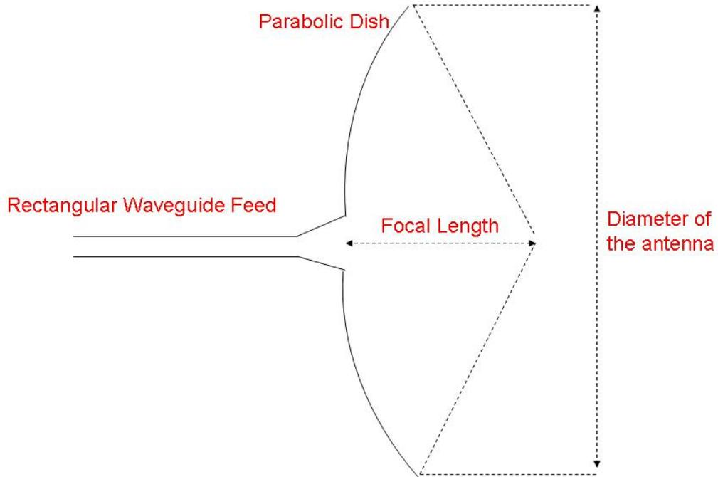
Figure 20. Aperture details of the proposed parabolic dish antenna
